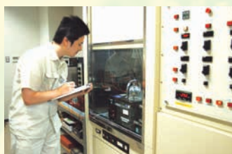
本質安全防爆電気機器の火花点火試験 Spark ignition test of intrinsically safe explosion-protected electrical equipment
