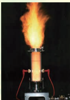
粉じん爆発危険性評価試験 Hazard evaluation test of dust explosion
